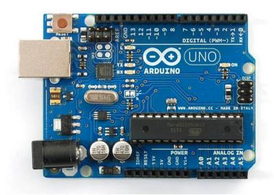
**Arduino** is the microcontroller development board that's taken the DIY world by storm. Adalight uses an Arduino Uno connected to a USB port to shuttle data between the host computer and the lights.
