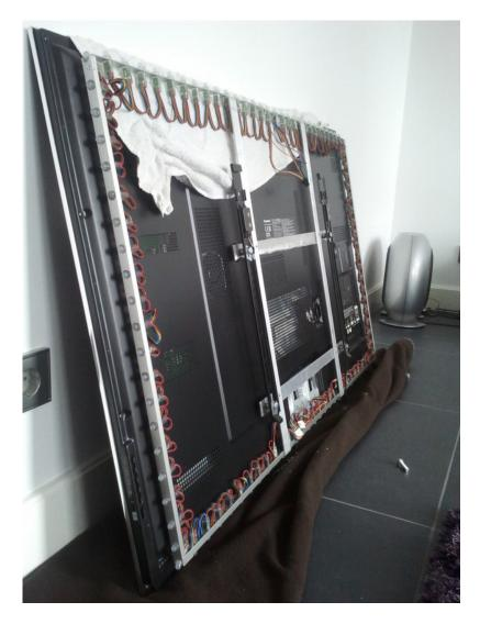
Forum user "Wackid" made this stunning <u>100 LED</u> Adalight frame using aluminum U-track with drilled holes carefully spaced around the perimeter. *Extreeeeme!*
