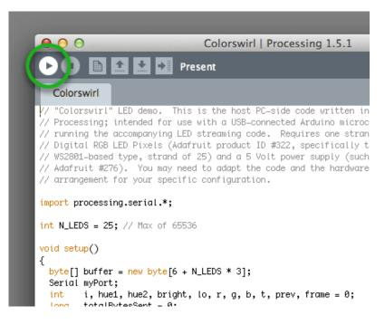
If the Arduino is the first or only serial device on the system, this should start a colorful rainbow of animation on the LEDs.
