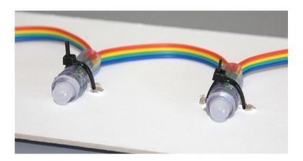
Cable ties work well with pixels on their side. Holes can be made using an awl, or you can make very clean holes using a leatherworking punch.
