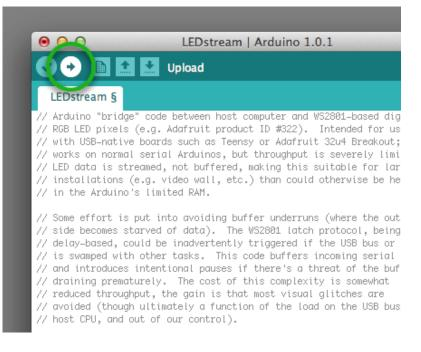
After the code is uploaded, if the LEDs are correctly wired up and the power supply is plugged in, the LEDs should all flash red, green, then blue for about a second each, then off. This is a startup diagnostic that tells you the LEDs and Arduino are working correctly, and are now awaiting data from the computer...
