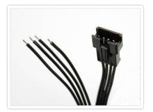
Alternately, if you don't want to use the "jammed wires" trick, an optional mating connector is available in the Adafruit shop (http://adafru.it/579). This has a plug housing at one end and four tinned wires at the opposite end...strip a little more insulation to press these into Arduino pin sockets.
