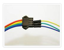
You can press wires directly into the plug connector. This works best with breadboarding jumper wires or solid-core (not stranded) copper wire.
